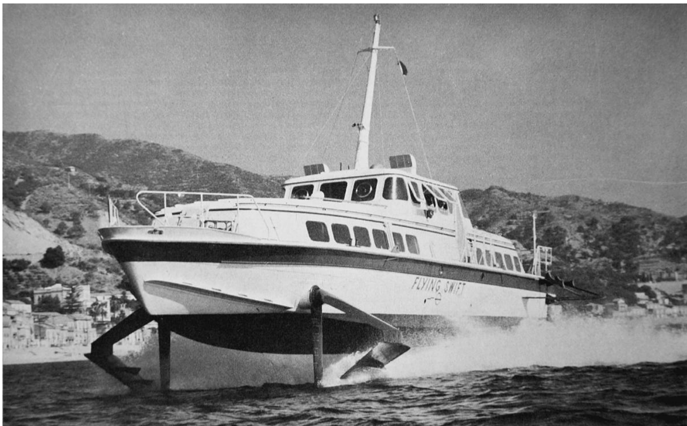
Above : Flying Swift was the third PT.20 delivered to HMH, in 1964. Note the covered up windows forward in the passenger saloon (also on Flying Kingfisher on page 4) / RODRIQUEZ CANTIERE NAVALE photo
