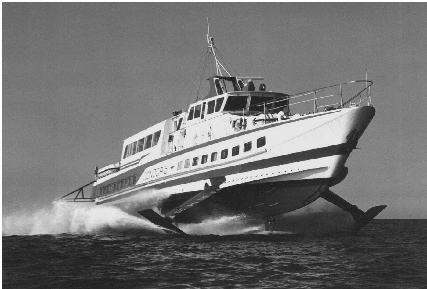
Above : Condor 5 as delivered to Channel Islands operator Condor in 1976. Supporting struts to the forward foil were subsequently fitted ( compare to Alioth on page 7, etc. ) The vessel, as in the case with Diomedea , was initially ordered by Hongkong Macao Hydrofoil / KEVIN LE SCHELLEUR photo
