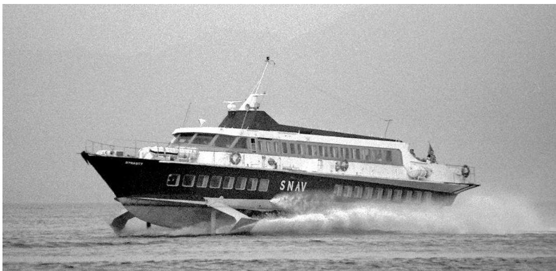
Left : RHS 150F Dynasty entered service with Aliscafì SNAV in 1984. It later operated for a short while in the Caribbean before returning to Italy and SNAV. The two production craft that followed were given the designation RHS 150M. The design is easily confused with the RHS 160F in its Australian version (see back cover), / TIM TIMOLEON photo
